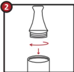
Filling of the tank: Please unscrew the black mouthpiece counterclockwise and subtract it. Then pour liquid into the tank to the upper scale. Put the mouthpiece back on the vaporizer and screw with some clockwise turns.
