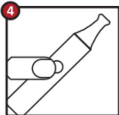
**Push and hold the release button of the battery and pull up the mouthpiece at the same time. Steam develops only if you press down continuously on the release button while drawing.**
