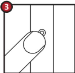
The battery of your red kiwi cLea is equipped with transport protection against accidental discharge, and in the as-delivered condition is switched off. To turn the transport protection on or off, press the button three times within two seconds.
