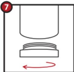
**7** To charge the battery, gently screw it into the round opening in the USB charger in a clockwise direction. Connect the USB cable either directly to a PC or a 220 volt or 12 volt USB adapter (both sold separately).
