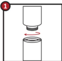
Screw the vaporizer into the battery with a clockwise turn. Please ensure that the threads are not crossed, as this may damage them.
